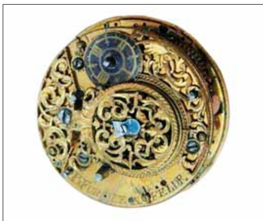
Fig. 2. The top plate of the Fürstenfelder with balance cock pierced in early eighteenth-century style. Photo courtesy of Mick Krening.
