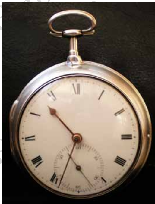
Fig. 1. Pocket chronometer 912, made by J A Mangaar. Diameter over the paired cases 63 mm, over the stem and bow as well 86 mm.
