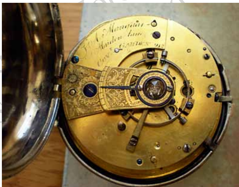
Fig. 4. View of the movement showing the large diamond end stone on the balance cock.
