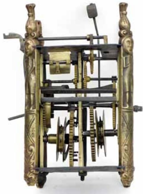
Fig. 6. Movement from the left. The winding click on the going greatwheel was removed during conversion to Huygens' loop.
