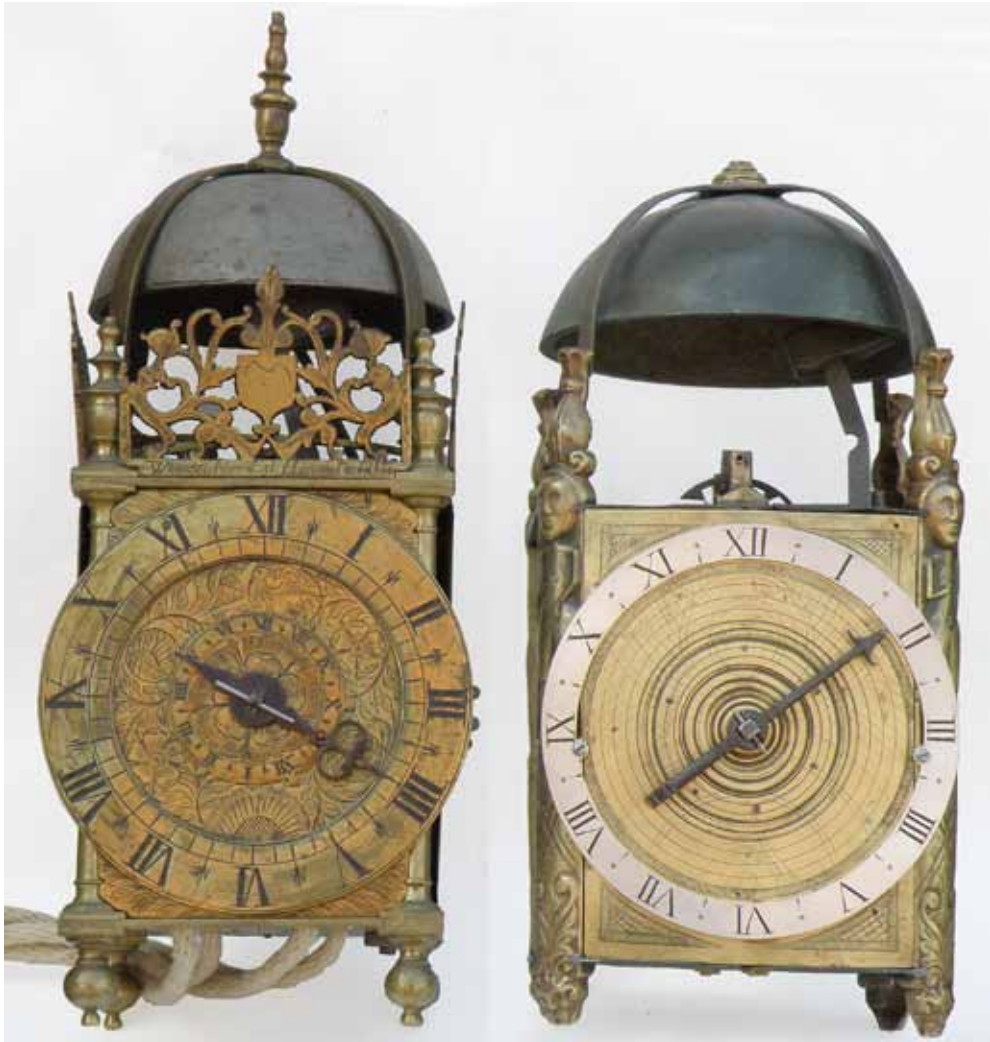
Fig. 2. The clock with its bell and restored chapter ring and hand (right). The frets are missing. Compared to a standard-size London clock by William Selwood from the 1640s (left), the clock is wider and due to the short feet appears to be squatter.
