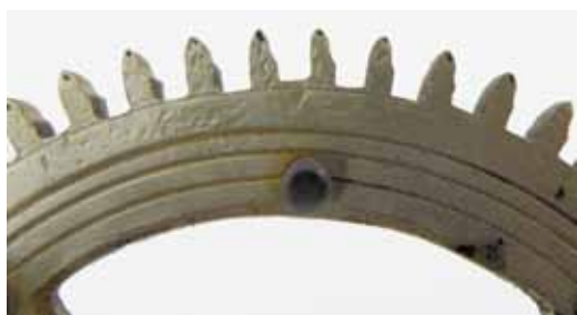
Fig. 8. Teeth of the greatwheel have considerable wear. The punch marks on the tips show that the teeth were marked out with a dividing plate before being cut and rounded by hand.
