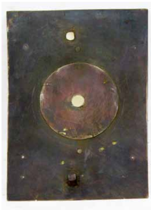
Fig. 14. Rear of the dial with the insertion of a thicker central section.
