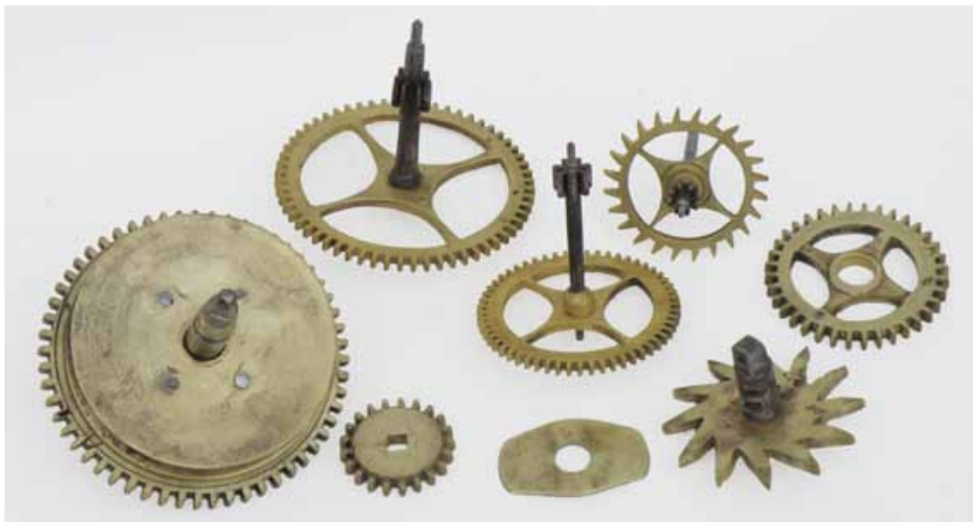
Fig. 10. The four wheels of the going train after conversion to long pendulum and anchor escapement, together with the starwheel and later pinion of report and hour wheel.
