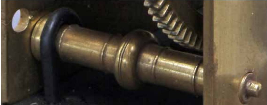
Fig. 8. The four finely fluted pillars with ringed knobs are screwed into the backplate – the pillar extensions on view from the back, are also ringed.
