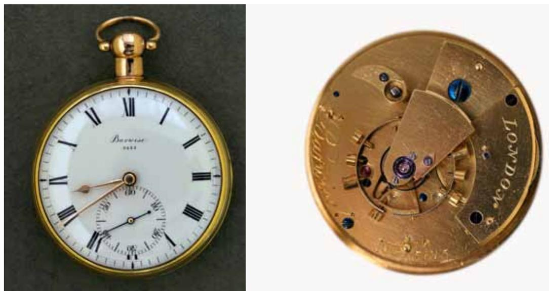
Fig. 8. Dial and back plate of a gold pocket chronometer signed *Barwise London* N<sup>o</sup> 5445. Back plate diameter 44.0 mm. Balance diameter 19.0 mm. Case diameter 54.8 mm. Total weight 151 g. Case maker T.H. Hallmark for London 1812. Private collection.
