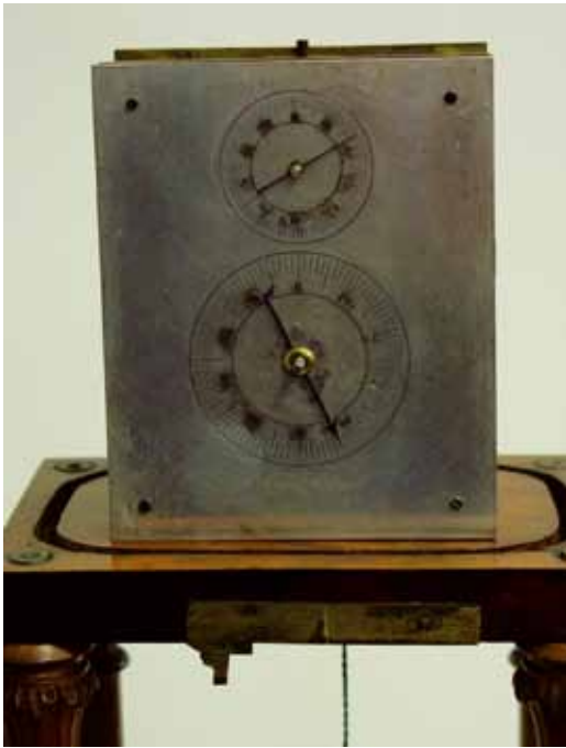
Figs 12 and 13. Front and back of the oldest surviving Hipp chronoscope, signed 'M. Hipp in Reutlingen' (1849). Utrecht University Museum, Inventory No. ME-30. Photos by Jan Deiman.
