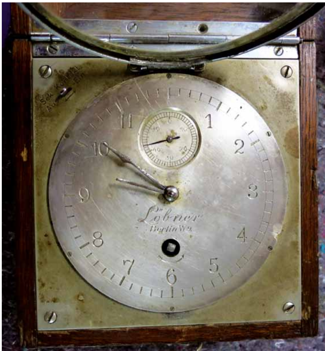
Fig. 4. Recently discovered, extremely rare Löhnner impulse clock, providing seconds input to the zeitdrucker , c.1936/37, as an alternative to a chronometer. Photo by the author.
