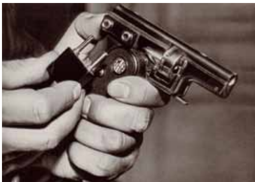
Fig. 6. Electric starting pistol, used at the Olympic Games in 1936.
