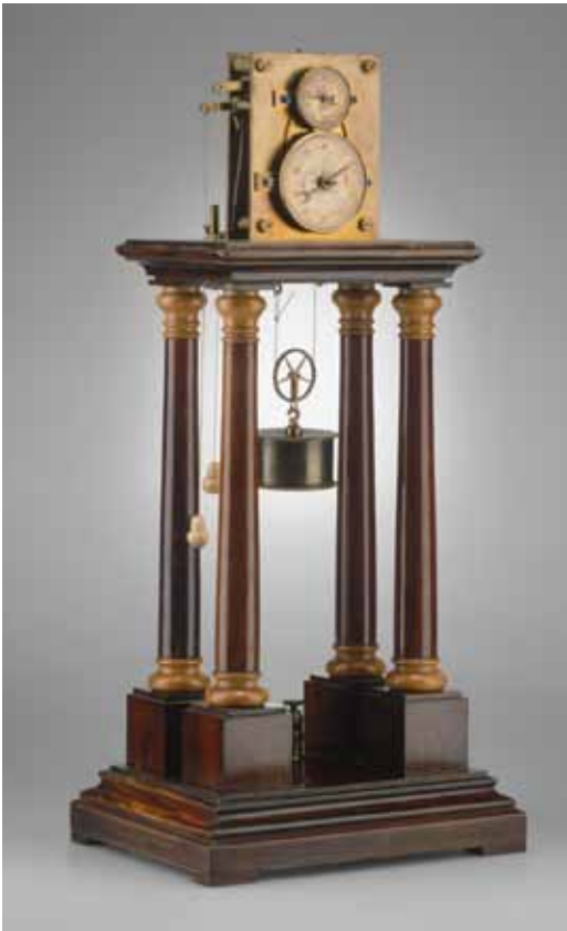
Fig. 14. Factory produced chronoscope, listed in Hipp's catalogue as model 75. Hipp No. 2889, c.1869. Photo Klaus Luginsland/Landesmuseum Mannheim.
