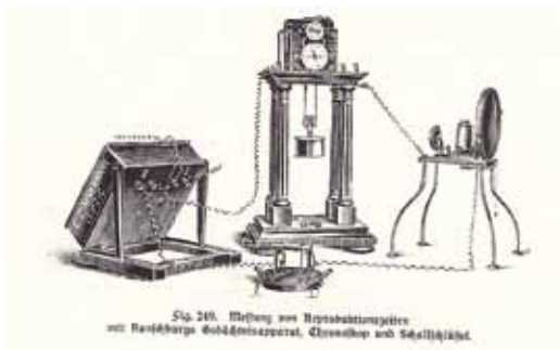
Fig. 30. Psychological experiment with Hipp chronoscope, memory apparatus and acoustic apparatus. See note 31 for source.
