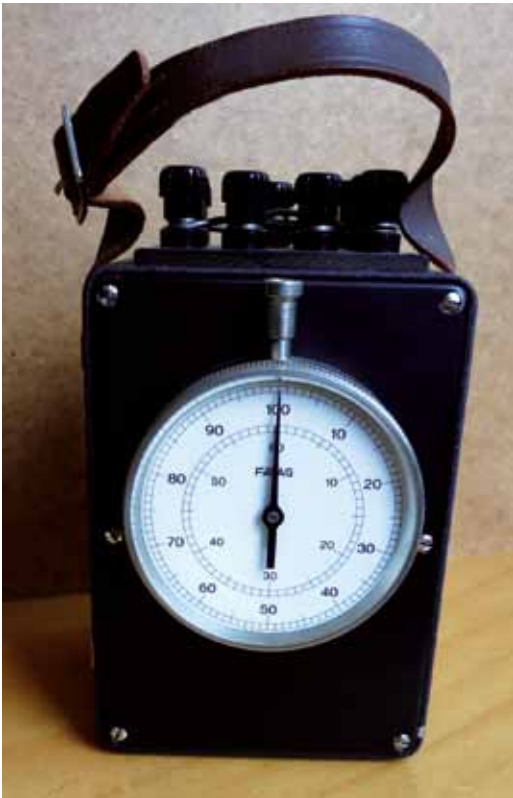
Fig. 18. Motor-driven Chronoscope 591974, 1959, by Favag Neuchâtel. Photo by the author.
