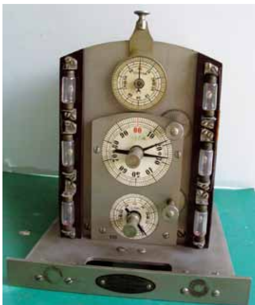
Figs 23 and 24. Special chronoscope with a time-switch driven by a synchronous motor. The maker was Joh. Hammer in Leipzig, c.1940. Most likely military use. Photos by the author.
