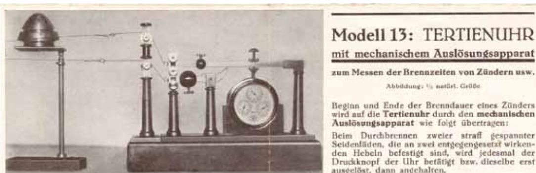
Fig. 10. Tertienuhr with mechanical release mechanism to measure the duration of burning of fuses etc. Undated catalogue 'Chronoskop und Tertienuhr', F.L. Löbner, c.1928.
