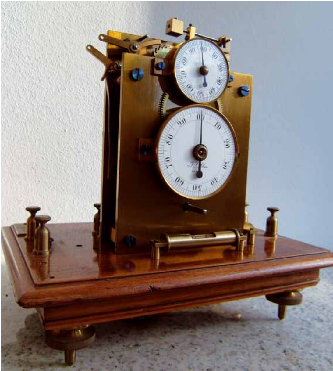
Fig. 21. Hipp chronoscope with a special contact sold by F.L. Löbner Berlin, c.1910. The maker was probably Strasser & Rohde from Glashütte. Photo by the author.
