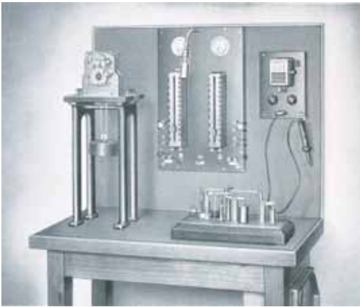
Fig. 28. Very accurate electric measurement of the burning time of gunpowder with a chronoscope. Joh. Hammer catalogue (c.1940).
