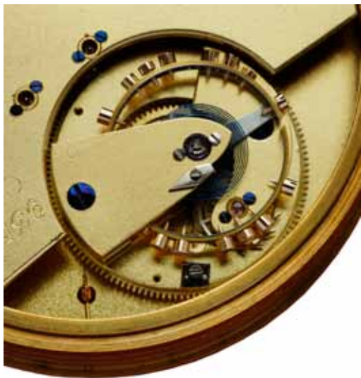
Fig. 9. The karrusel carriage of No.93539. The foot of the spring detent can be seen in the lower part of the image.
