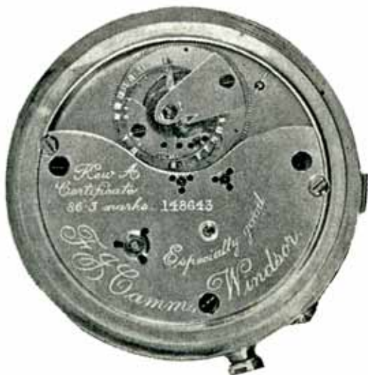
Fig. 4. The F.J. Camm centre seconds karrusel watch as illustrated in his book Watches Adjustment and Repair .
