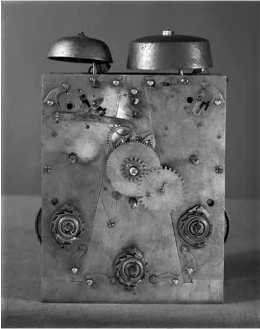
Fig. 8. Print from Negative 8 - Front Plate Movement View of a Joseph Knibb Table Clock.
