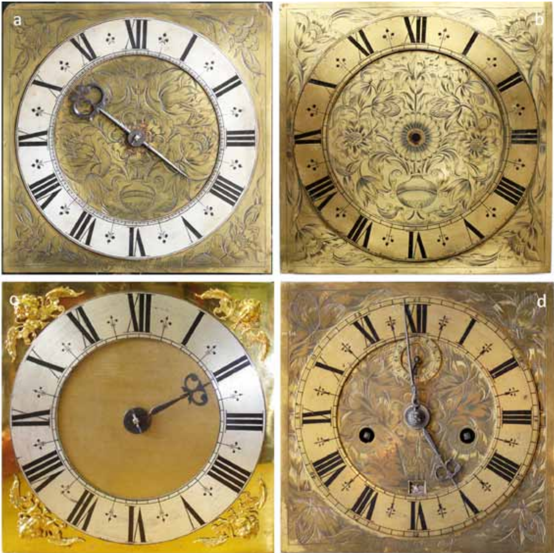
Figs 1a-d. Dials of the signed 30-hour Knibb (a), D&H (b), the 30-hour Abraham Fromanteel (c) and the 8-day Abraham Fromanteel (d). There are traces of remaining fire gilding on the D&H and 8-day dials. The signed 30-hour Knibb dial is 9\frac{3}{8} in (239 mm) square, has chapter ring, 1\frac{5}{8} in (34 mm) with 8\frac{1}{2} in (215 mm) external diameter. The D&H dial is 9\frac{3}{8} in x 9\frac{1}{4} in (251 mm wide x 253 mm high) with 1\frac{1}{2} in (32.4 mm) chapter ring of 8\frac{7}{8} in (226 mm) external diameter. The signed 30-hour Knibb dial is very thin.
