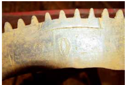
Fig. 7. The repair in the year 1423: a dovetail insertion of four teeth, performed by Maestro Paolo ingeniero (engineer) from Venice. In the wheel numbers are scratched from 5 to 60 in units of 5; their significance is unclear.
